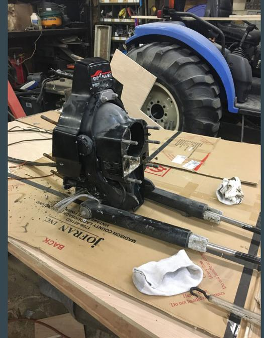
Cleaning up outdrive and replacing anodes to prevent corrosion
