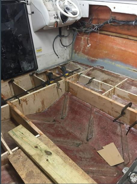
Installing new homemade stringers(floor supports)
